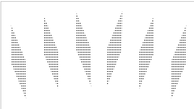
Figure 3-79 Angle shape with dash and pattern; caps and join ignored
